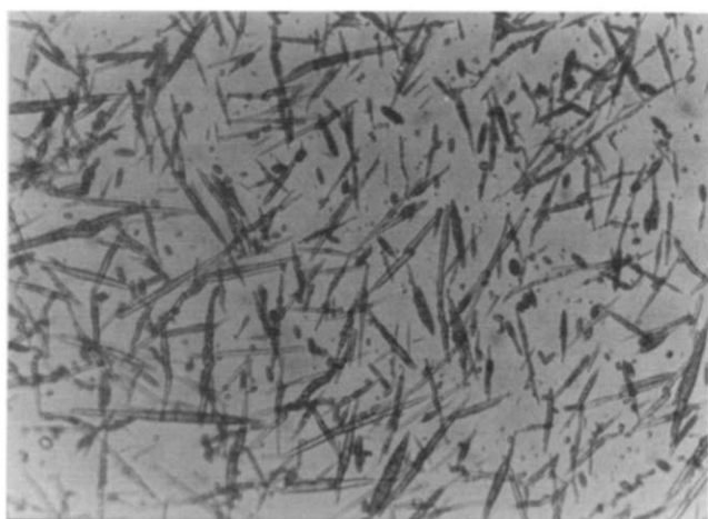
Figure 5 Hot-stage photomicrograph ( \times 267 ) of a drawn sample [PP/LCP (wt/wt) ratio 100/10]
